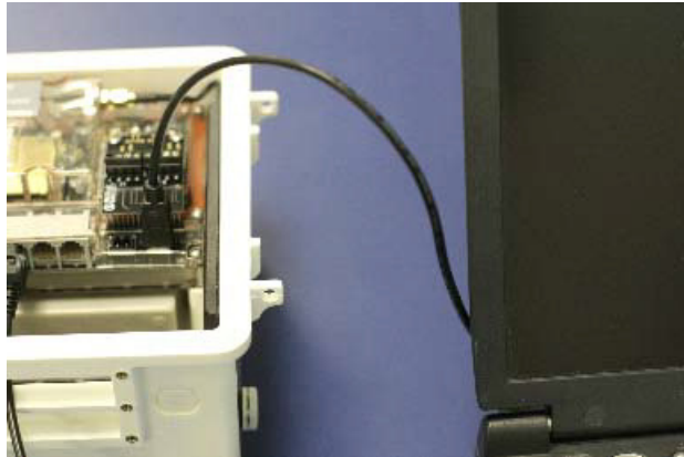
Figure 8: Connecting the U30 to a computer
