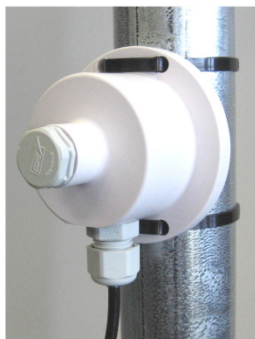
Figure 1: S-BPB Mounted to Tripod Mast
