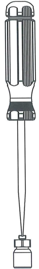
FIG 5: IF FOR ANY REASON THE MOUNTING STUD DOES NOT DISENGAGE FROM THE SENSOR, USE A FLAT HEAD SCREW DRIVER TO HOLD THE STUD WHILE TURNING THE HEX NUT COUNTERCLOCKWISE WITH A WRENCH.
