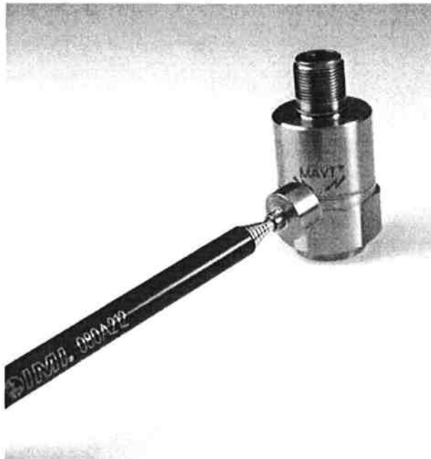
Touch magnet to MAVT™ point on the Smart Vibration Switch
