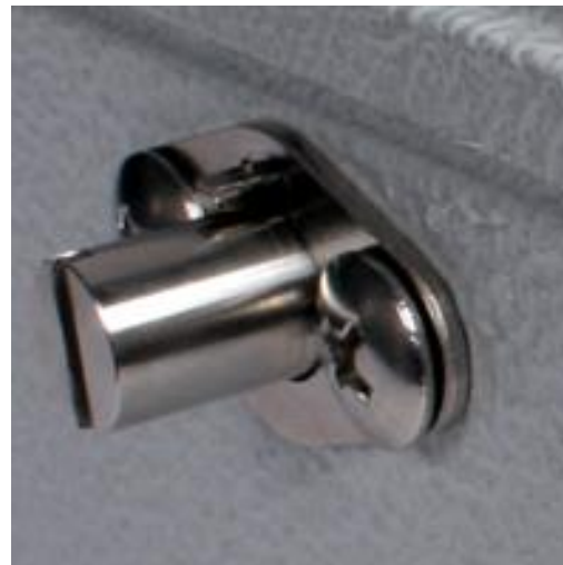
Figure 2: Sensitivity Adjustment Screw
