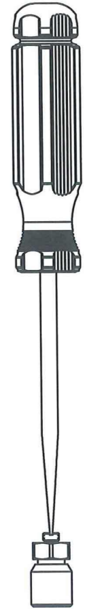
FIG 5: IF FOR ANY REASON THE MOUNTING STUD DOES NOT DISENGAGE FROM THE SENSOR, USE A FLAT HEAD SCREW DRIVER TO HOLD THE STUD WHILE TURNING THE HEX NUT COUNTERCLOCKWISE WITH A WRENCH.
