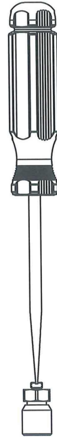
FIG 5: IF FOR ANY REASON THE MOUNTING STUD DOES NOT DISENGAGE FROM THE SENSOR, USE A FLAT HEAD SCREW DRIVER TO HOLD THE STUD WHILE TURNING THE HEX NUT COUNTERCLOCKWISE WITH A WRENCH.
