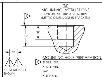
THREAD DEPTH: B= X + 1 THREAD PITCH DRILL DEPTH: C= B + 3 THREAD PITCH SEE A-F FOR APPROPRIATE DRILL AND TAP THREAD PITCH= 1/TPI [P]
