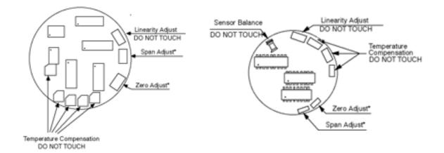
NOTE: When circuit cover is removed, a zero shift can be noticed. The zero will return by the same amount when the cover is replaced. This displacement of the output should be taken into account when making adjustments or during recalibration
