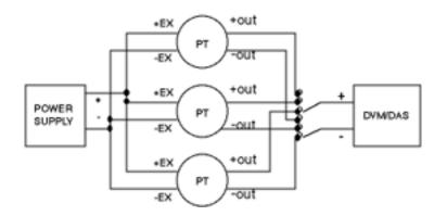
NOTE: The shield is internally commoned to the case and pressure port of the transducer. When the shield is connected to ground the case and pressure port of the transducer will also be commoned to that ground.
