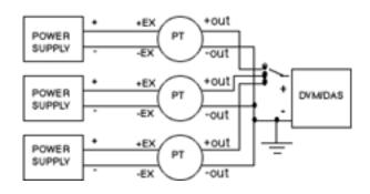
Power Supply (Nominal 24 VDC) PT - Pressure Transducer (4 Wire Circuit) DVM/DAS - Digital Volt Meter or Data Acquisition System
