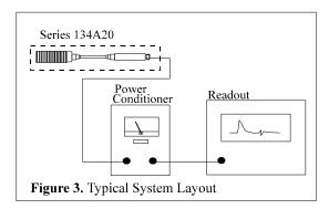
Tie the three-inch, low-noise cable to a rigid structure to prevent excessive motion and noise. Allow for strain relief.
