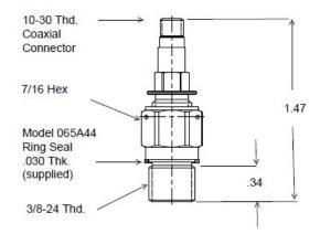
Series 102B10: Cryogenic Pressure Sensor
