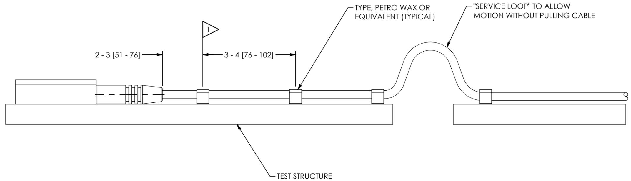
1 FASTEN CABLE TO TEST STRUCTURE TYPICALLY WITHIN 2-3 [51-76] OF SENSOR, THEN FASTEN AGAIN WITHIN 3-4 [76-101] OF PREVIOUS ATTACHMENT, BETWEEN THE TEST STRUCTURE AND A FIXED STRUCTURE, ALLOW A SERVICE LOOP LARGE ENOUGH TO PREVENT PULLING OF THE CABLE WHEN SHAKING, MORE ATTACHMENT POINTS WILL PROVIDE LESS NOISE IN THE RESULTING DATA, LOOSE CABLES OR PARTS ELSEWHERE ON THE TEST STRUCTURE CAN ALSO GENERATE "NOISE" ON THE SIGNAL RECEIVED FROM THE MODEL 3741 SERIES
