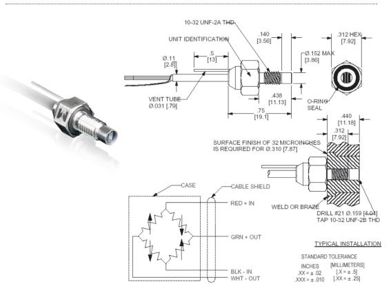
Model 8510B is a rugged, miniature, high sensitivity piezoresistive pressure transducer. It has a 10-32 mounting thread, 0.15 inch (3.8 mm) face diameter and is available in ranges from 1 psi to 2000 psi. High pressure ranges are shown on this sheet. Its high sensitivity combined with high resonance makes it ideal for measuring dynamic pressure.
